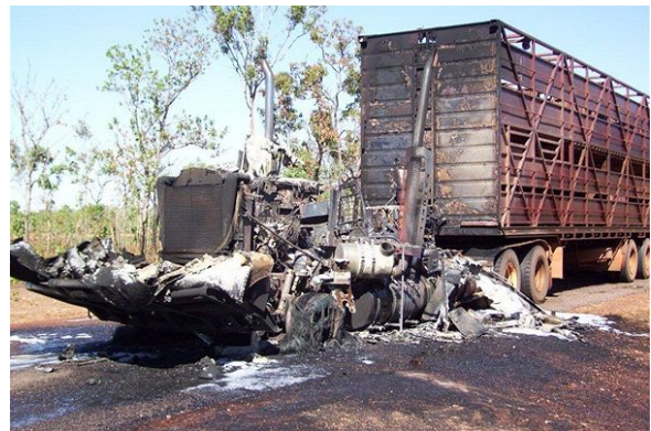
The road train cabin burnt to the ground, however the trailers were only scorched. | Photographer: | Margo Bellis
