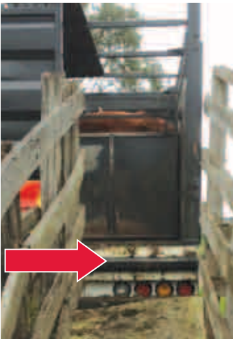
FIGURE 3b Note – Ramp not at suitable height.
