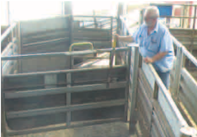
FIGURE 16a Externally operated gate at a commercial facility
