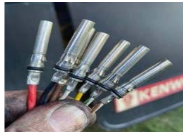
O-ring sealed EBS socket crimp terminals
