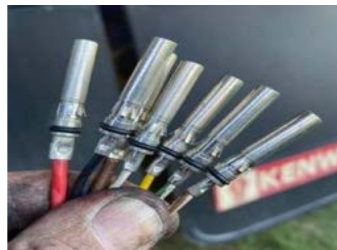
O-ring sealed EBS socket crimp terminals
