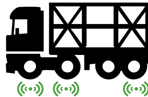
Instant electronic signal to every brake valve in the system.
