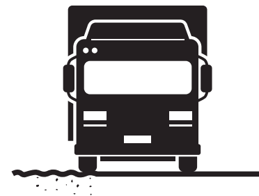
Braking when wheels face uneven friction, like one side leaving the pavement
